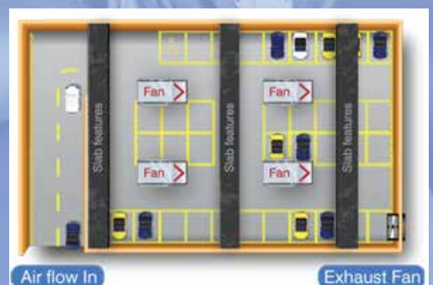
Figure 7(b). Fan's air movement perpendicular to beams is less effective
