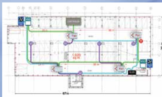
Figure 12. Fan sizing and placement example
