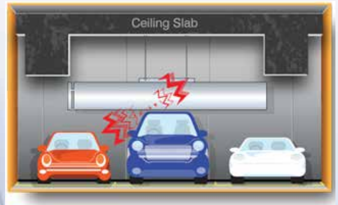
Figure 8(b). Insufficient clearance
